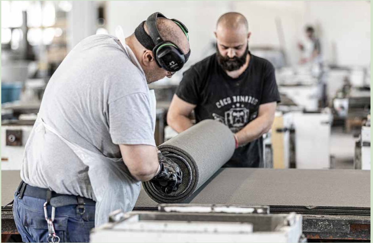
The moist, still moldable fiber cement mat is rolled onto the molded piece using a fine roller. After it is completely dry, the fiber cement shell is cured and the tub is ready for use.
