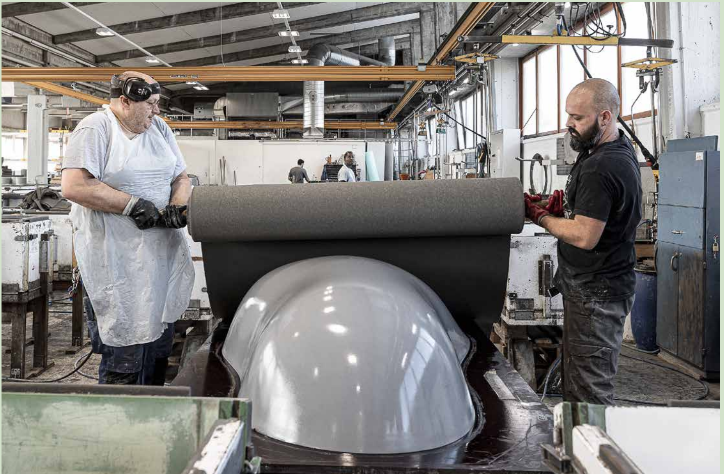
The moist, still moldable fiber cement mat is rolled onto the molded piece using a fine roller. After it is completely dry, the fiber cement shell is cured and the tub is ready for use.
