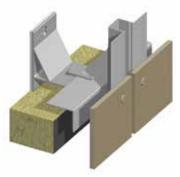
Attachment method with rivets. For use with flat panel products such as fiber cement, HPL or fiber concrete panels. Ideal for stud backup walls with panels in landscape orientation. Rivet attachment guarantees high pull-out values and ease of installation.
