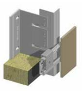
Attachment method with undercut for cement composite, ceramic, stone, HPL and fiber concrete panels. The back of each panel is predrilled using undercut drill bit to receive the hanger clip and expanding bolt anchor.
