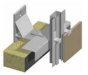
Attachment method with visible clips. Costeffective visible clip attachment system used for anchoring ceramic or natural stone panels for cladding applications. Clips are color matched to the panels and are discreet, especially for multiple story construction. For use with either stud or concrete back-up conditions.
