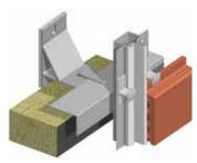
Concealed clip fixing for double-skin terracotta tiles. Designed for TC30 and TC40, double-skin terra-cotta tiles, to limit water penetration and provide a mechanic clip solution for attachment. Clips are concealed in the tile ship-lap. For use with either stud or concrete back-up conditions.
