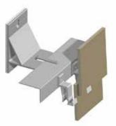
Semi-concealed clip fixing for lap-siding applications. Unique clip system devised for fixing fiber cement, ceramic, HPL or fiber concrete panels in a lap-siding configuration. Mechanically fastened clips and variable depth brackets with simple horizontal L-profiles make this system an economical solution for lapsiding applications.
