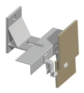
Semi-concealed fixing for lap-siding applications. Unique clip system devised for fixing fibercement or HPL panels in a lap-siding configuration. Mechanically fastened clips and variable depth brackets with simple horizontal L-profiles make this system an economical solution for lap-siding applications.
