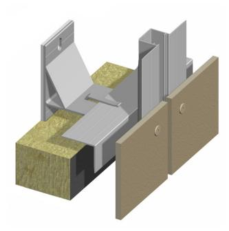
Attachment method with rivets. For use with flat panel products such as SwissPearl® cement composite, HPL or fiber concrete panels. Ideal for stud back-up walls with panels in landscape orientation. Rivet attachment guarentees high pull-out values and ease of installation.
