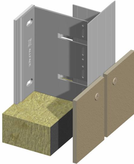
Attachment method with rivets. For use with flat panel products such as cement composite, HPL or fiber concrete panels. Ideal for concrete substrates with panels in landscape orientation. Rivet attachment guarantees high pull-out values and ease of installation.
